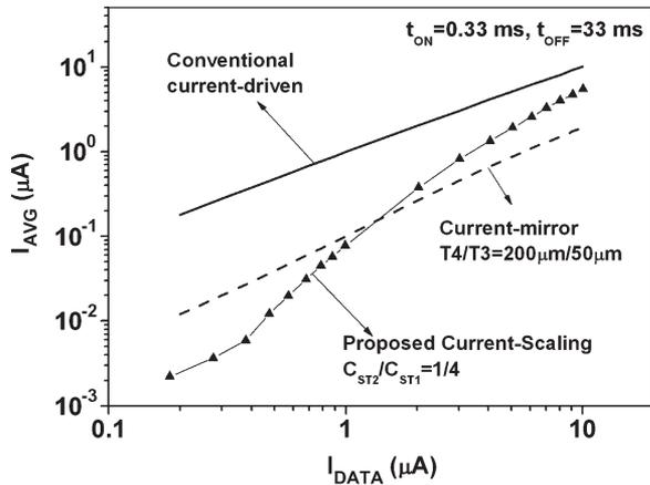
Fig. 6. Comparison of  $I_{AVE}$  versus  $I_{DATA}$  for conventional current-driven, current-mirror, and proposed pixel circuits.
