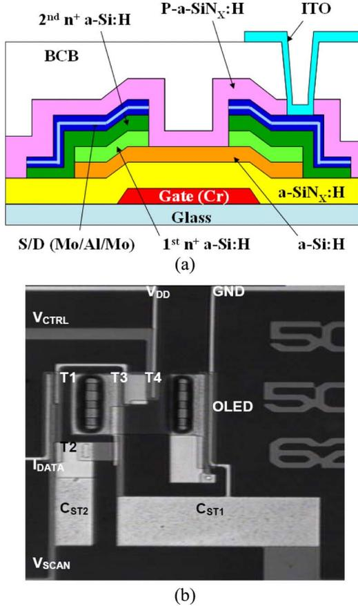
Fig. 1. Schematic cross section and top view of the fabricated a-Si:H TFT pixel-electrode circuit.
