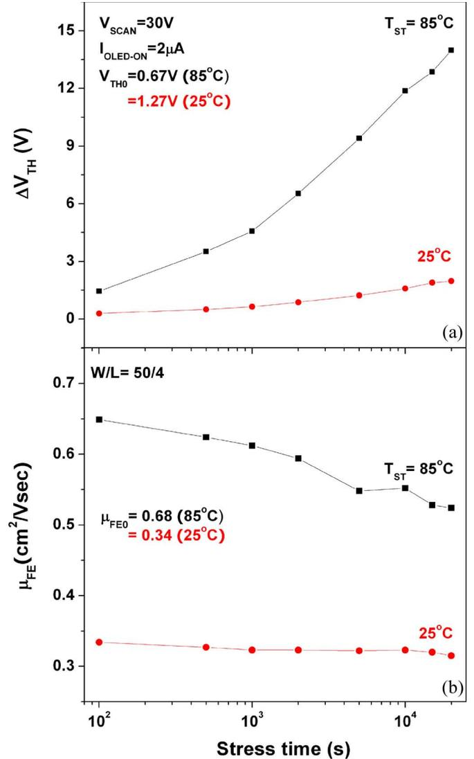
Fig. 9. Variations of threshold voltage and field-effect mobility of a-Si:H TFT ( $W/L = 50/4$ ) as a function of stress time at  $25^\circ\text{C}$  and  $85^\circ\text{C}$ .
