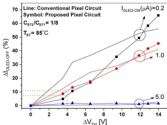
Fig. 10. Variations of the OLED OFF-current ( $\Delta I_{\text{OLED-OFF}}$ ) of the proposed pixel circuit as a function of threshold-voltage shift ( $\Delta V_{\text{TH}}$ ) at 85 °C in comparison to the conventional current-driven pixel circuit.
