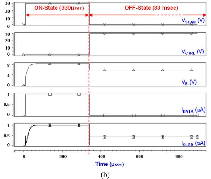
Fig. 2. Schematic of (a) cascaded-capacitor pixel-electrode circuit and (b) operational waveforms simulated by HSPICE.
