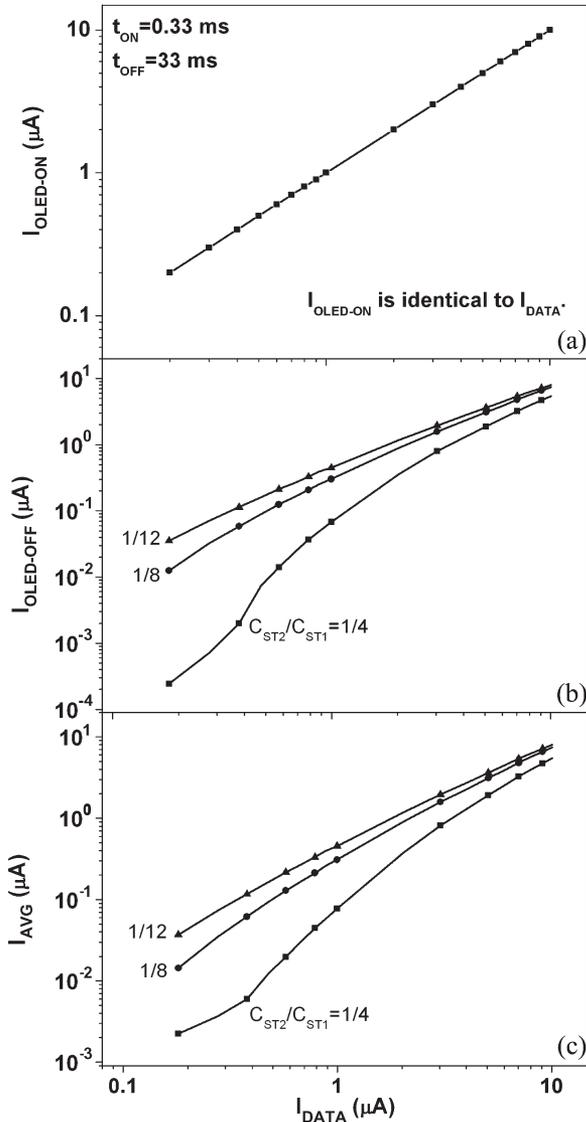
Fig. 3. Variation of the measured  $I_{\text{OLED\_ON}}$ ,  $I_{\text{OLED\_OFF}}$ , and  $I_{\text{AVE}}$  as a function of  $I_{\text{DATA}} (= I_{\text{OLED\_ON}})$  for various  $C_{\text{ST2}}/C_{\text{ST1}}$  ratios.
