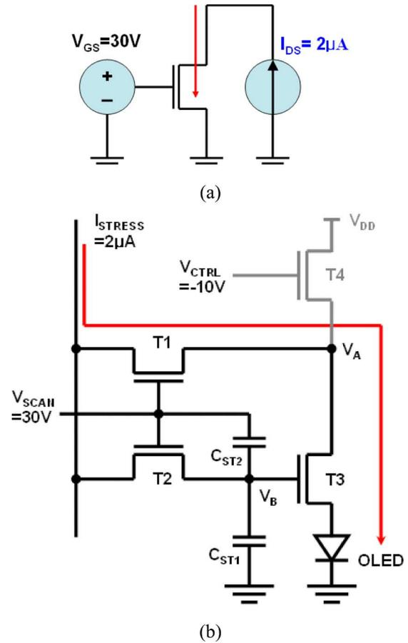
Fig. 7. Schematics of the CTS measurement setup used for (a) single a-Si:H TFT and (b) proposed pixel-electrode-circuit stability study.
