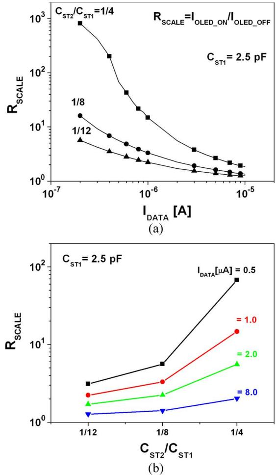
Fig. 4. Variation of the measured current-scaling ratio as a function of (a)  $I_{\text{DATA}}$  and (b) ratio of storage capacitances for fabricated cascaded-capacitor pixel circuit.
