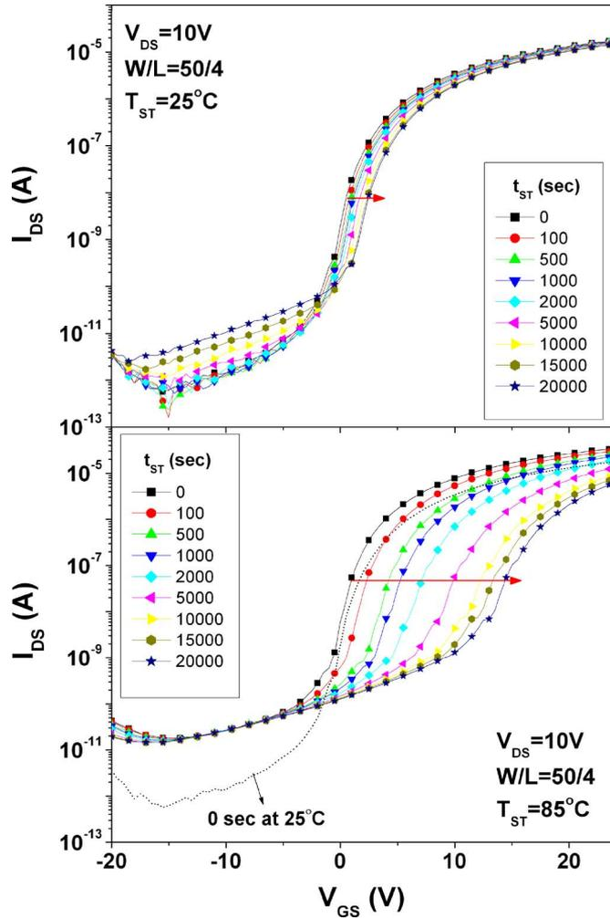
Fig. 8. Transfer characteristic of TFT ( $W/L = 50/4$ ) after current-stress ( $I_{\text{DATA}} = 2 \mu\text{A}$ ) as a function of stress time (a) at room temperature ( $25^\circ\text{C}$ ) and (b) at  $85^\circ\text{C}$ .
